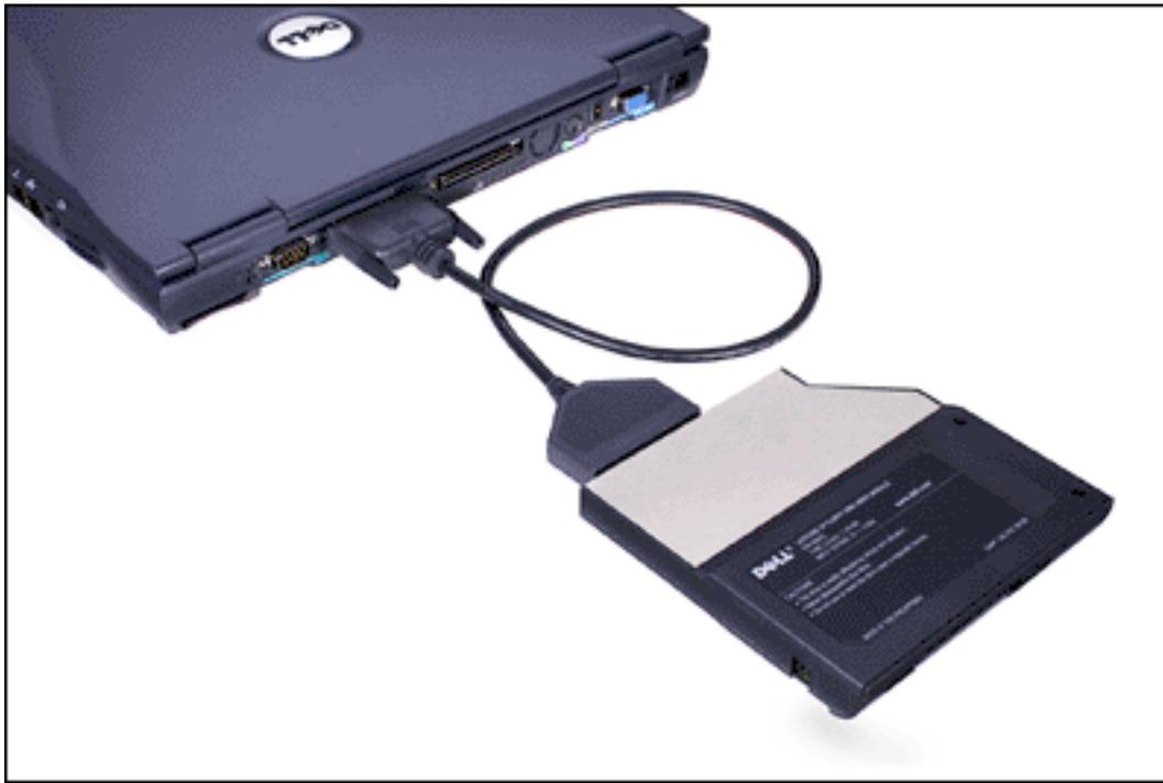
**NOTICE:** When the diskette drive is not being used externally, remove the parallel diskette-drive cable from the parallel connector.
